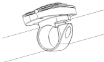
4. Use one M3\*10 screw and M2.5 internal hex wrench to tighten the control pad onto the handlebar. Torque requirement: 1N.m.
